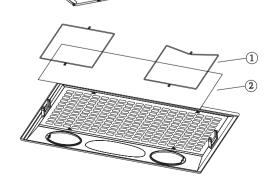
replacing the paper grease filter.
